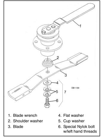
Figure 11. Blade Installation & Removal
